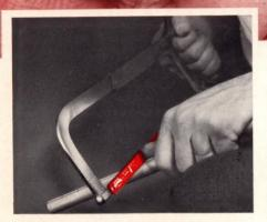
New blade cuts so easily that pipe, tubing, thin sheet, electrical conduit, etc., can be handheld and thumb-guided to a line or mark.
