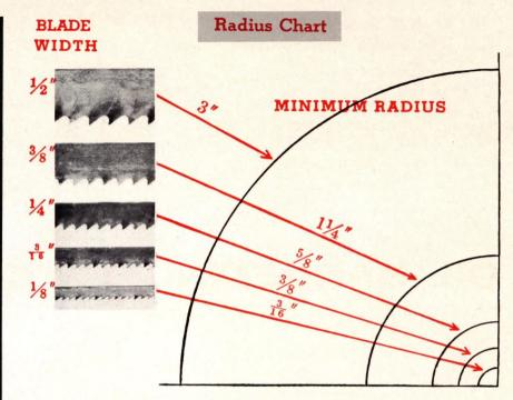
In contour sawing the radius of the curve to be cut governs the width of the saw to be used. The smaller the radius, the narrower the blade. For desired radius use width of saw as indicated by above chart.
